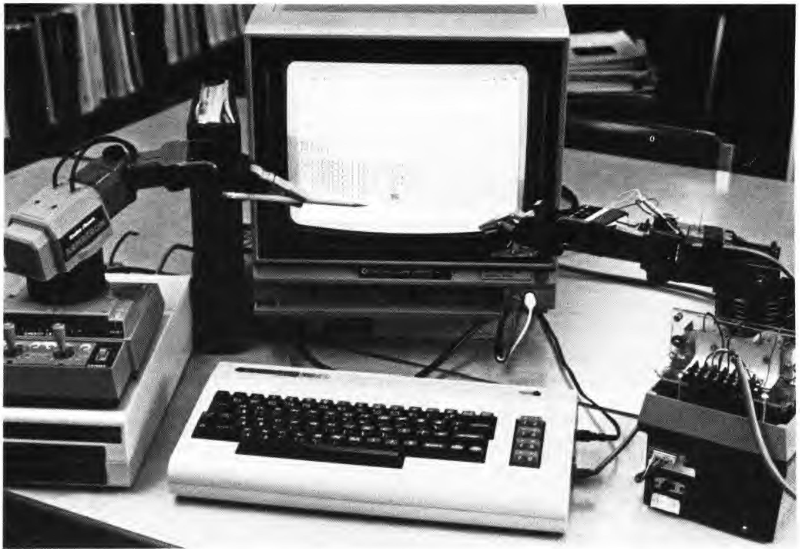
Figure 1. Armatron Robot Arms. The left model on top of the disk drive is unmodified and shows the two joysticks for control. At right the modified robot arm sits on top of the power supply and interface box.
